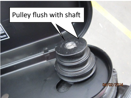
15. Fit the Motor Pulley, making sure the key is in place. Tighten the grub screw.
