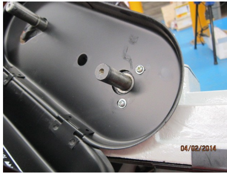
14. Using these 2 screws and 1 bolt, fit the Belt Guard as shown.
